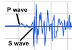
What is the **Time difference** ( $\Delta T$ ) between the P and S waves? \_\_\_\_\_
