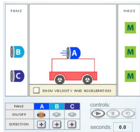
By blowing to the left, the fans exert a **force** on the cart that pushes it to the right. This illustrates **Newton's third law**: A force in one direction results in an equal force in the opposite direction.
