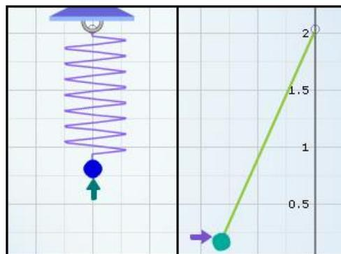
1. When the spring touches the arrow, click the green button on the stopwatch. Count the movements, or **oscillations**. Click the green button again after the tenth oscillation.
