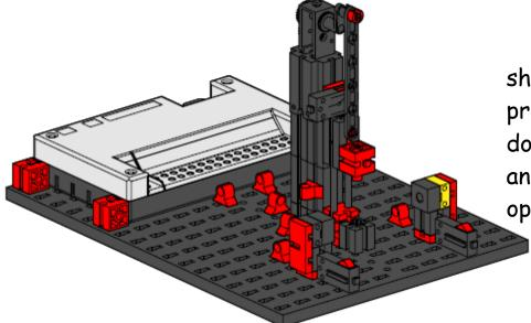
Build and program a sheet metal stamping press machine using a double startup switch and a light beam for safe operation.
