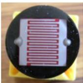
**Photo Sensor** - detect changes in the amount of light. Using an analog branch, photo sensors must be calibrated to respond to the specific light range needed. Photo sensors are wired into the **AX terminals** of the computer interface.
